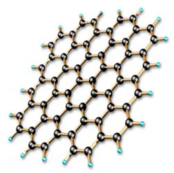
Carbon atoms form graphene in a hexagon pattern resembling chicken-wire
